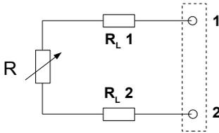
This is the simplest way, but line resistors (RL1 and RL2) are connected to the sensor in a series circuit. The addition of RL1 + RL2, leads to an off-set between measured temperature and real temperature. This connection must be avoided.
